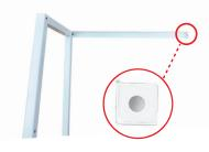
Secure **Link Rod - Back** in the top hole on the back of **Left Frame** with an M6 screw.
