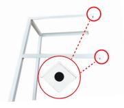
Secure 2 **Link Rod - Front**, into the top 2 holes on the front of the **Left Frame**.
