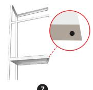
Fasten a **Top Shelf** to the **Left Frame** using 2x **M6 Screws** in the next set of holes below the 2nd **Link rod - Front**.
