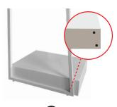
Working from the bottom of the frame to the top, take a **Bottom shelf** and attach to the bottom holes of the **Left Frame** using 4x **M6 Screws**.
