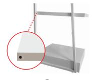
Next, fasten a **Middle Shelf** to the **Left Frame** using 2x **M6 Screws** in the next set of holes.
